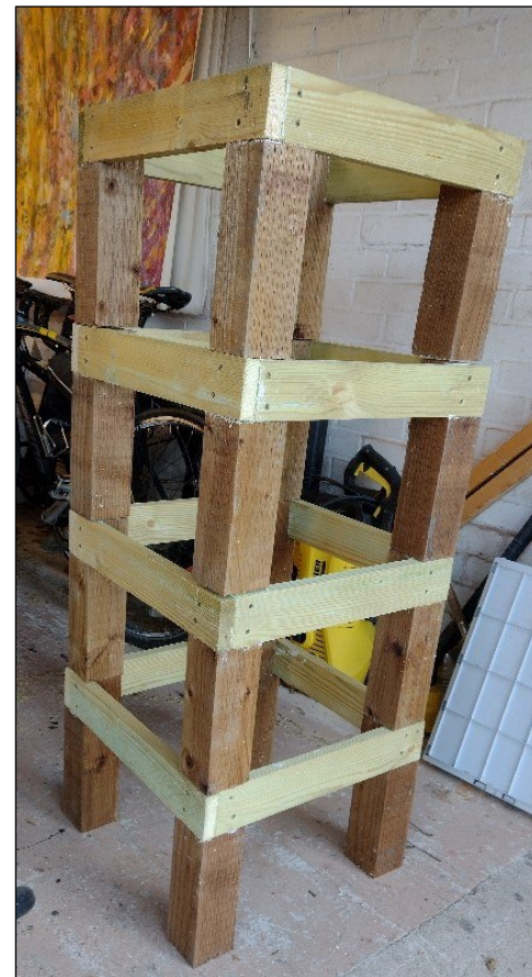
(right) Four completed single hive stands. The legs are just 300mm tall. Each fence post gave eight pieces.
